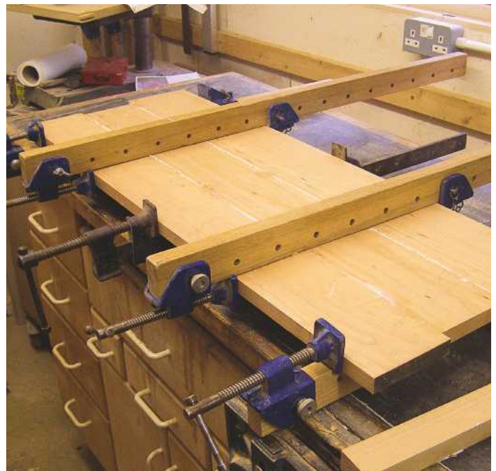
▲ Pic.3 Cramp the boards together, alternating each side to equalise the cramping force
